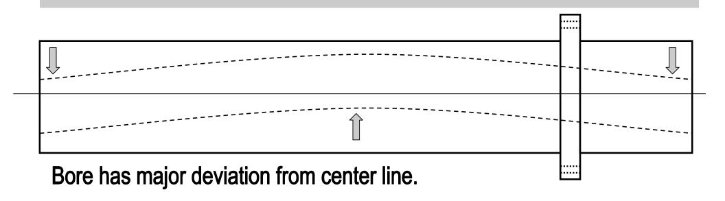
Screw to barrel contact shown by arrows.
