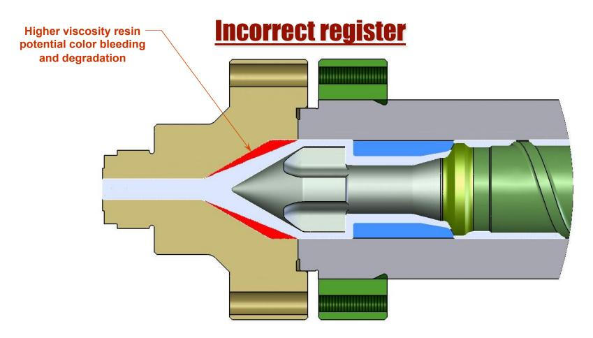
Excessive cushion. Besides increasing viscosity, material that remains in the cushion area can increase the potential for residual stress, color bleeding, and degradation
